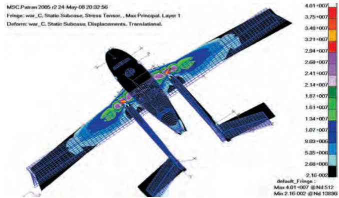
Fig. 14d — Distribution of the primary stresses after static analysis for the C-case: extreme stress \sigma_{\max} = 40.1 MPa
