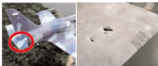
Fig. 1 — Damage of aircraft structure after impact of a military projectile
