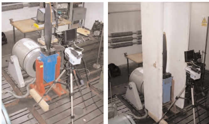
Fig. 1 — Composite propeller blade mounted in a special fixture for excitation of the first three natural vibration modes. The thermographs were taken using a thermal insulating box
