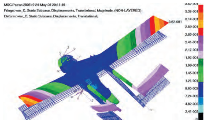
Fig. 14b — Distribution of the node displacements after static analysis for the C-case: u_{\max} = 362 mm
