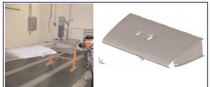
Fig. 5 — Measurement of real aircraft structure after damage
