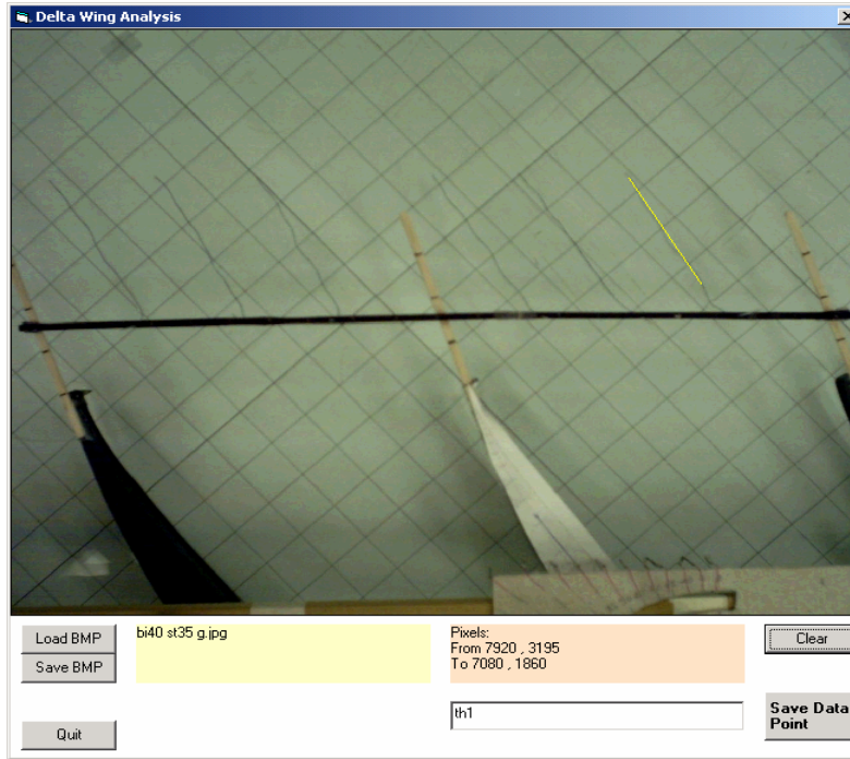
Figure 7 – Computer assisted data analysis window screen shown with a yellow line highlighting angle for tuft #1.
