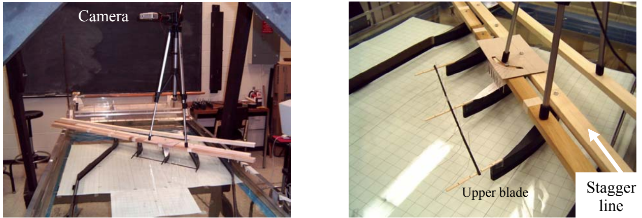
Figure 5 – Water table cascade set-up with grid lines, view from downstream (left) & view from upper blade (right).
