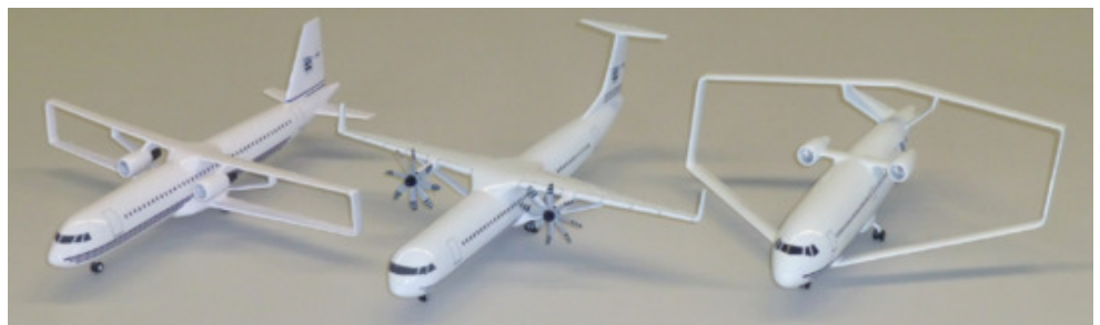
New aircraft design concepts. Smart turboprop (center) and boxed wing aircrafts (left and right).
