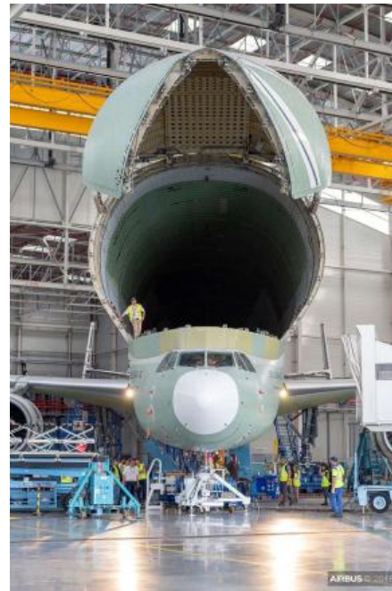
Main cargo door and cargo loading system concepts similar to Beluga ST designed for compatibility with existing infrastructures
