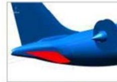
CROR design study: interference with HTP
