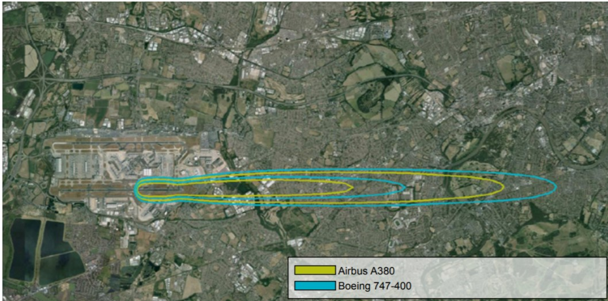
Figure 5.6 Airbus A380 noise contour during arrival (85 dB(A)) and departure (90 dB(A)) in comparison to Boeing noise contour (CAA 2014)
