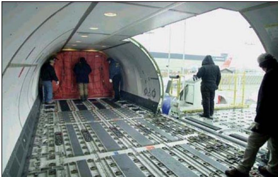
Fig 6.1 B757 Side Door Loading ( Massachusetts Institute of Technology 2004 cited in Vrydag 2007 )
