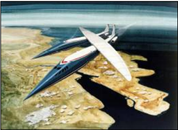
Fig 2.16 Twin-Fuselage Oblique Wing Transonic Transport Aircraft (Hirschberg 2005)
