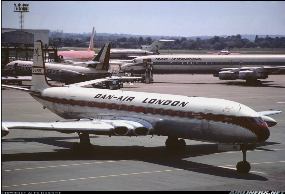
Fig 3.12 Engine Integration in Wing Root (de Havilland Comet, airliners.net 2007)
