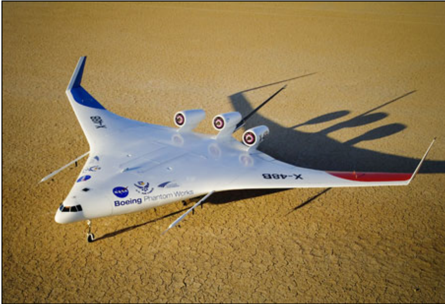
Fig 2.22 Picture of the Boeing X-48B Flight Model ( Flight International 2007b )
