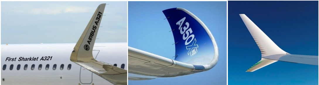
Fig. 1 – Different winglets on passenger aircraft: A321 Sharklet [1], A350XWB Blended Winglet [2] and B737 MAX AT Winglet [3]
